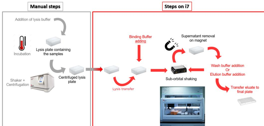
**Figure 1. Automated DNAdvance Extraction On Biomek i7 automated workstation Workflow.**
